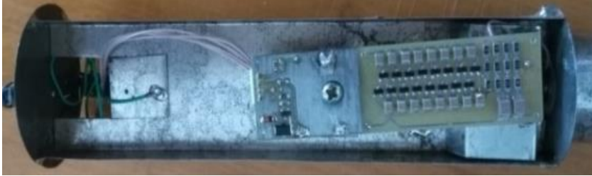
Figure – 4 the main connection nodes and signal transmission from the developed equipment for automatic measurement of neutron fluxes.
